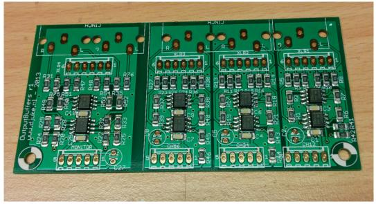
The result of my first attempt is shown in the picture above. All components are nicely reflowed, no bridges were seen around the ICs. The joints look smooth. I used lead-free solder paste, with a soak phase of 90s at 180 deg, then temperature was increased to 240 deg for reflowing. Visual observation showed that the solder paste started to reflow around 220 deg.
