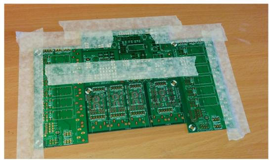
Photo shows some spare pcb to form a kind of mold to fit the pcb. The polyester stencil is hardly visible but is fitted on top of the pcb that will get the solder paste.
