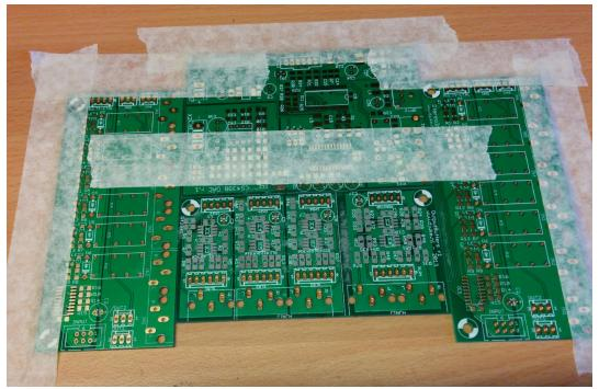
Solder paste is applied with an old bank card. Below shows how accurate this can be done.
