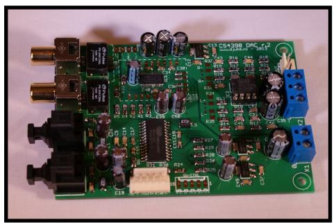
The photos on the left, top and bottom side show some examples of completed projects: a 100W stereo Mosfet amplifier, a digital-to-analog converter with 2 optical and 2 coaxial inputs and a modular multi-channel pre-amplifier with integrated media player (Volumio/Rune Audio/etc).
