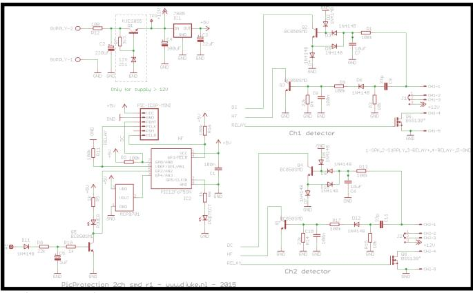
The functionality of the circuit is very similar to the modular version with through-hole components. As an additional feature, an onboard 12V supply is generated from the input voltage, which can be used to switch a 12V relay. Instead of a BJT, a FET is now used to switch the output relay. With the BSS138, max positive relay voltage is 50V (can be increased to 60V by replacing BSS138 with MMBF170).
