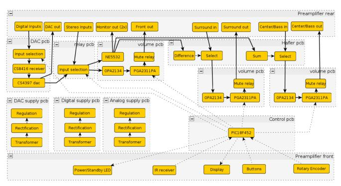
The different components and the signal flow are shown in the figure below.
