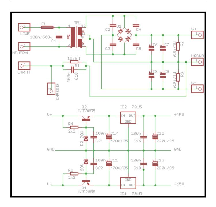
To achieve 100W in an 8 ohm load, 28.3Vrms or 40V peak is needed at the output. Due to the fact that a MOSFET output stage is used, about 48V rail voltage is needed to achieve this. Taking into account a 1V voltage drop in the rectifier, the needed transformer voltage is (48+1)/1.41 = 34.75V, so a dual 35V transformer would be about perfect. Most manufacturers of toroidal transformers specify their voltage rating under load, so the unloaded rail voltage will be some volts higher.
