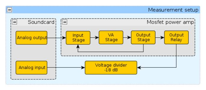
Because the output voltage of the mosfet amp is far too high to be connected directly to the analog input of the sound card, I used a simple voltage divider to attenuate this signal. This has some influence on the measurement results, especially the measured bandwidth, which seems lower, because the analog input of the sound card is not driven from a low impedance source anymore. THD and noise measurements are not influenced very much.
