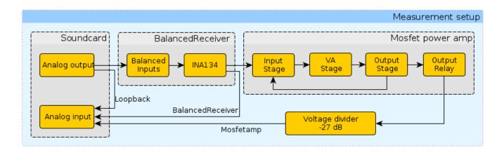
At three positions in the chain, the results are measured:
