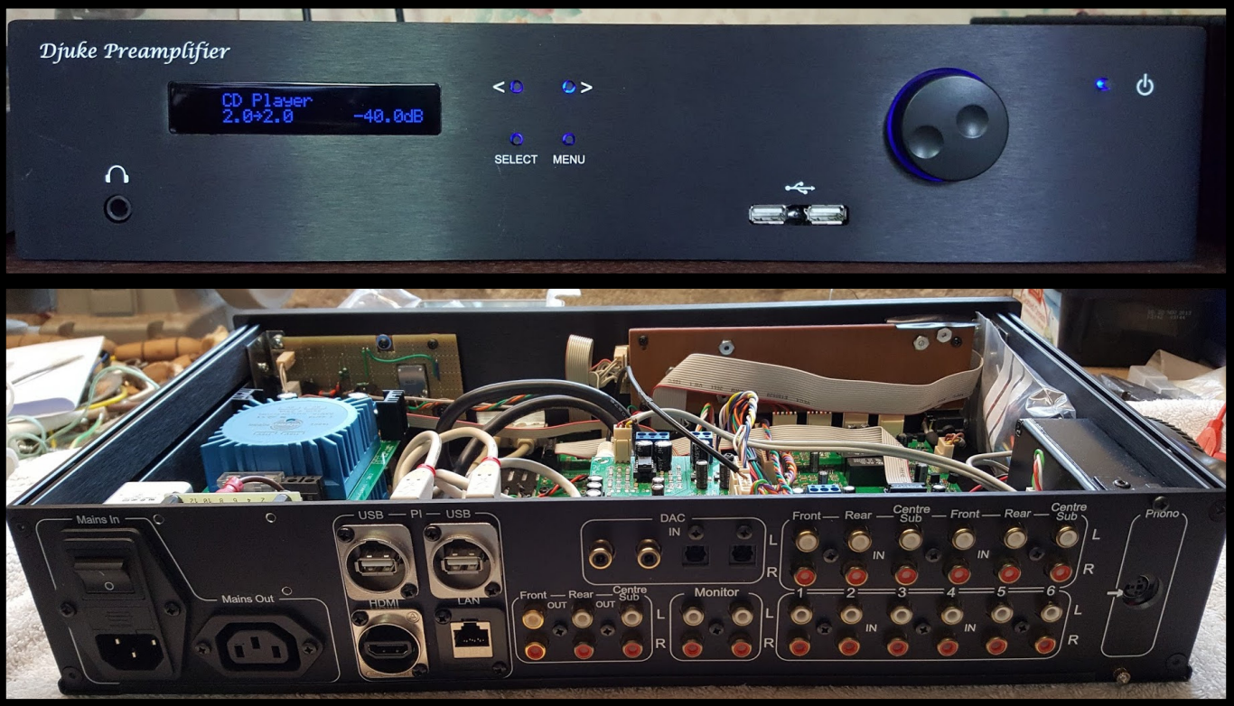
Peter Bellamy Fully featured 5.1 channel amplifier built inside a custom enclosure. Also includes a third party phono preamplifier.
