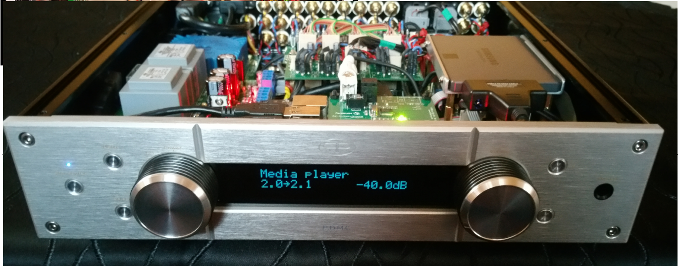
Full 5.1 preamplifier with CS4398 DAC and Raspberry Pi media player built inside a custom cabinet
