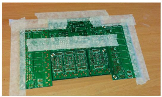
Photo shows some spare pcb to form a kind of mold to fit the pcb. The polyester stencil is hardly visible but is fitted on top of the pcb that will get the solder paste.
