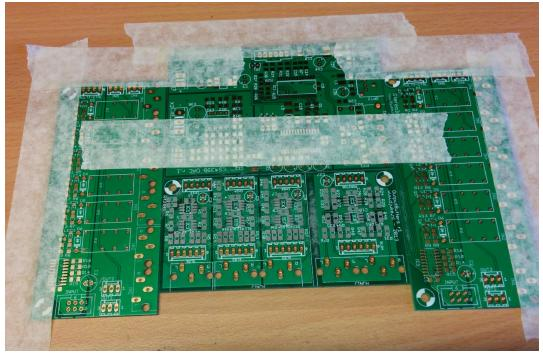
Solder paste is applied with an old bank card. Below shows how accurate this can be done.
