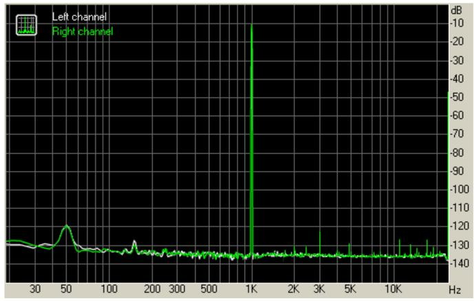
The result is quite amazing. The THD goes down to 0.0004% which is really a remarkable value. Actually, the DAC output measures better than the output stage of the E-MU 1212m card I used for measuring it.
